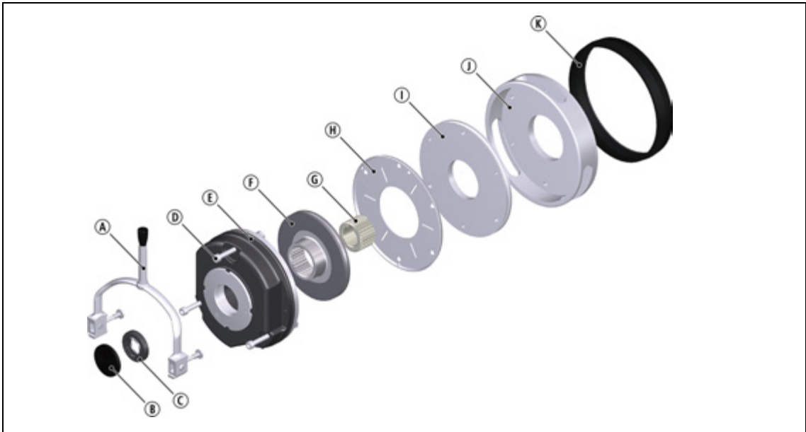
Fig. 32 Spring-applied brake INTORQ BFK458-06 to 25
