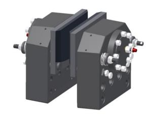
Two springs on each brake half retract the brake pads from the disc when pressure is released. Brake lining wear is automatically compensated for with increased piston stroke.
