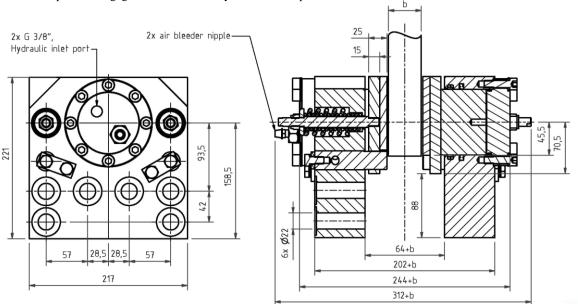
b = Brake disc thickness
