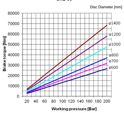
The braking torque is calculated from the following formula:
