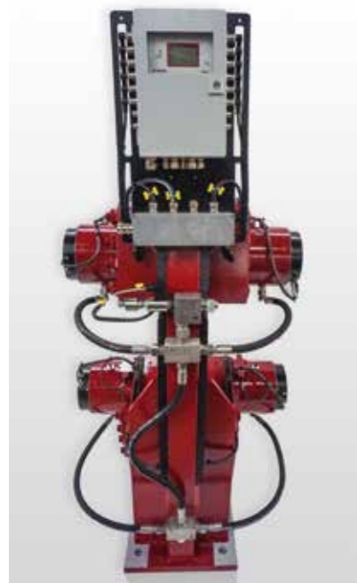
Brake type: Two SF24 on console with one CMB3.
