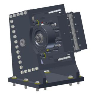
In order to compensate for friction pad wear and to maintain full brake capacity, the spring pack must be adjusted a few times during the life span of the friction pad. The unique, well proven Dellner Brakes design, with an extension of the brake piston through the cylinder provides an easy visual way to tell when adjustment is needed. As an option, the brakes can be equipped with proximity switches to indicate brake ON/OFF, PAD WEAR and/or NEED OF ADJUSTMENT.
