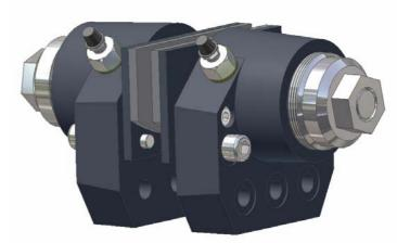
Each brake half has two cylindrical guide pins that transmit the tangential braking force from the brake lining to the brake housing and support. As a result, any radial forces on the brake pistons are minimized which contributes to longer brake life.
