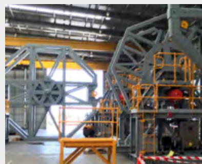
Mining conveyor belt reeler, Australia
