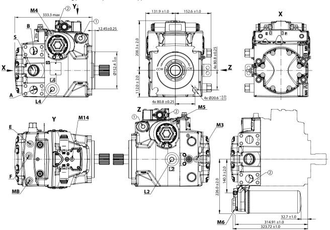
**A/B** system ports: Ø31.5 mm; M12 x 1.75; 20 min. full thread depth; Recommended screw in depth 1.5 x thread dia
