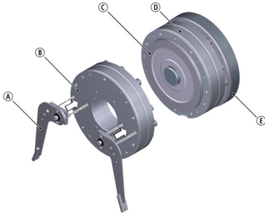
Fig. 17: Applying the hand-release lever
