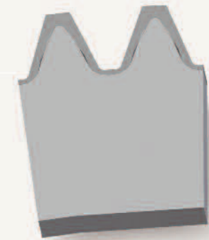
induction hardening of tooth side and bottom
