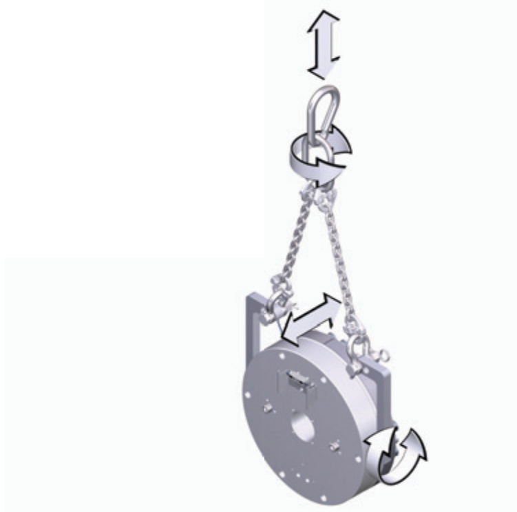
Fig. 8: Lifting mechanism for hooking onto a hoist
