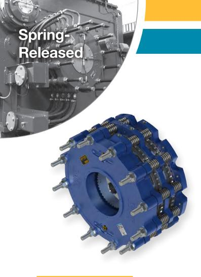
WPT® Water Cooled Brakes (WCB) are a high energy absorbing solution used for dynamic tensioning. The design of the internal water flow and copper alloy wear plates allow for excellent heat dissipation. WCB's are well suited for applications where a heavy-duty continuous slip tensioning is needed such as drawworks, mooring winches, dynamometers, paper converting, uncoilers and yarders.
