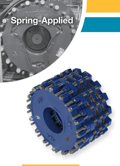
WPT® Water Cooled Spring Applied Brakes are a high energy absorbing solution used as a dynamic tensioning, static holding, or emergency stop brake. These brakes are spring-applied and released through pneumatic or hydraulic pressure. The WCB Spring Applied Brake is ideal for applications that require dissipation of large thermal loads such as marine winches, drilling rig drawworks, and logging equipment.
